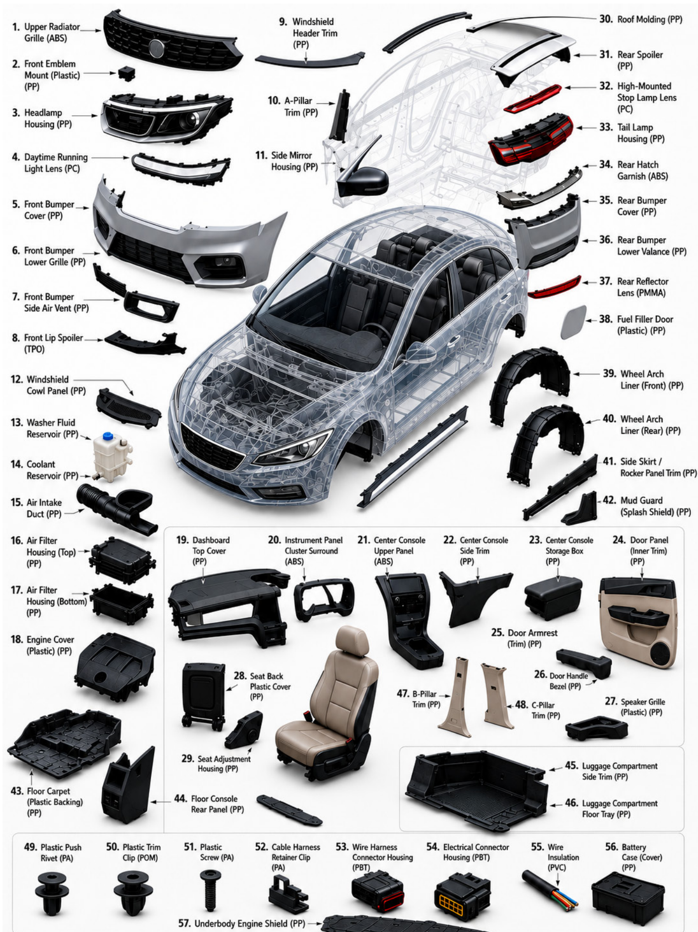
Figure 1. Plastic applications in automotive components. Material selection may vary depending on manufacturer, vehicle model, component design, and performance requirements.
